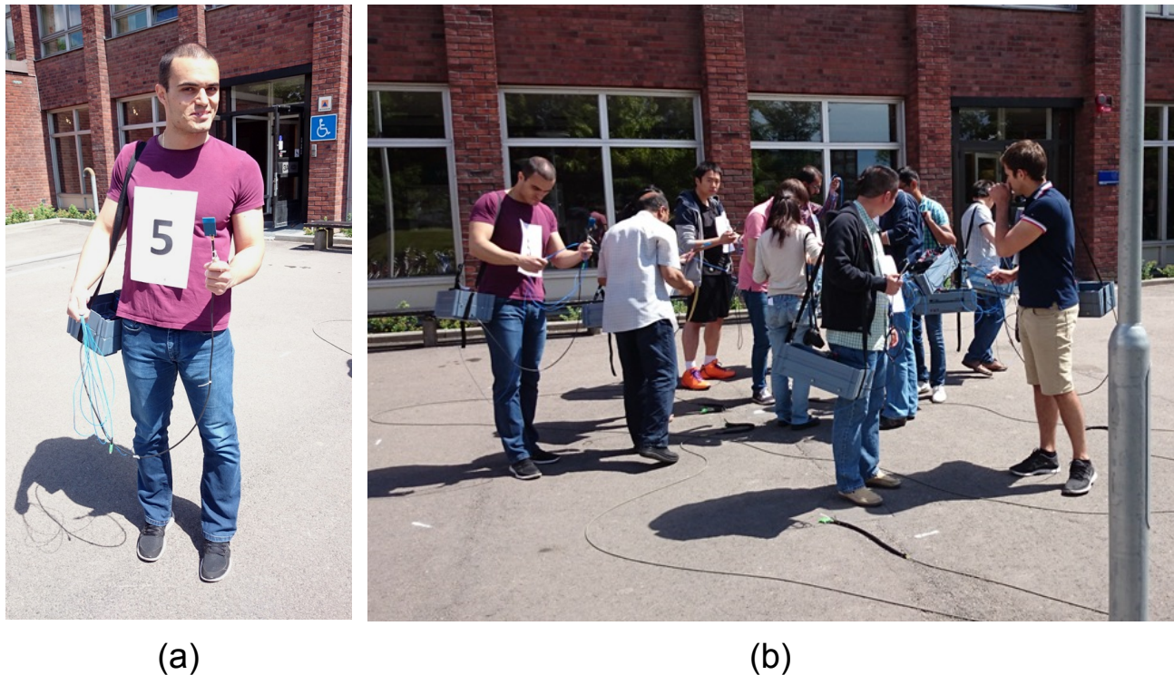
Figure 4.2: (a) A user holding the MS user equipment antenna with an inclination of 45^\circ . (b) Users moving randomly within the five-meter diameter circle.
