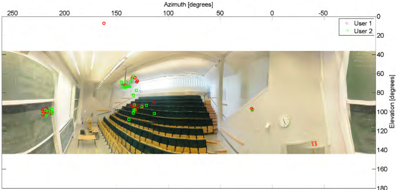
Figure 6.18: LOS component and the 30 strongest multipath components for users 1 and 2, at snapshot 10. This figure corresponds to an indoor auditorium deployment (BS 3, users at the back). There is LOS and no crowd is present.
