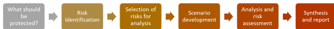
Figure 3: General process for assessments and reporting on national risks as developed in Sweden, redrawn from MSB (2011).
