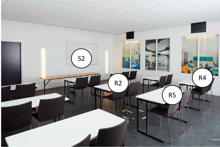
Figure 18 One source / speech position, S2, three receiver positions, R2, R4 and R5, used in the listening test.
