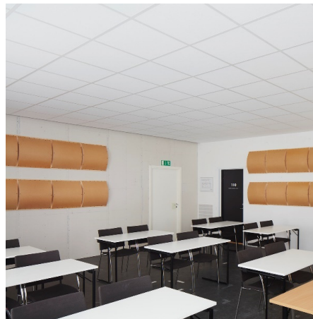
Figure 15. Diffusers, in all configurations, were mounted on two adjacent walls, as shown in this image. In each configuration, the same set-up was always used for the two walls.
