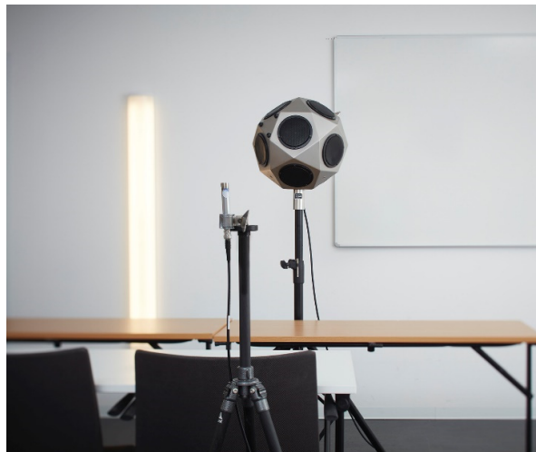
Figure 16. Loudspeaker and microphone used in the room acoustic measurements. The loudspeaker had its center at 1.50 m from the floor. The microphone was placed at a height of 1.20 m from the floor.
