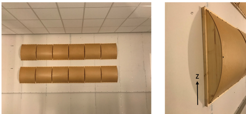
Figure 7. Vertically oriented diffusers, majority of reflections will be sent in z-direction.
