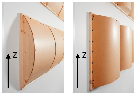
Figure 10 Diffusers used in the studies. Left picture: vertically oriented diffuser, directing majority of sound waves vertically. Right picture: Horizontally oriented diffuser, directing majority of sound waves horizontally.
