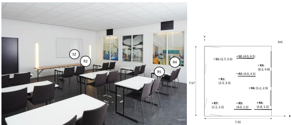
Figure 4. The positions used for sound sampling. The speech was emitted from S2 and sampled in R2, R4 and R5. In the sketch to the right, the positions used in sound sampling are underlined. All positions shown in the sketch were used for the averaged values of room acoustic measurements.
