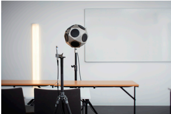
Figure 12 Loudspeaker with dodecahedron geometry and omnidirectional microphone in the mock-up room.
