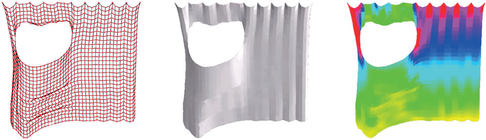
Figure 19: Different visualisations of a hanging cloth simulation. Each visualisation provides discernment of different aspects. Each of them are based on the same simulation, but they are visualised differently.
