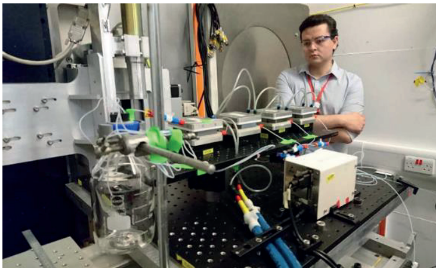
Figure 3.7. The INTER reflectometer at ISIS (Webster et al. , 2006) and the author of this report during an experiment presented in Paper IV (Orozco Rodriguez et al. , 2022c) of this report.
