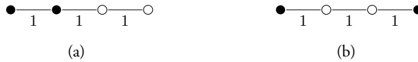
Figure 2.1: The cut values of the first partition (a) and the second partition (b) are respectively 8 and 6. It follows that single geometric cuts are not always sufficient to generate minimum bisections on the real line.
