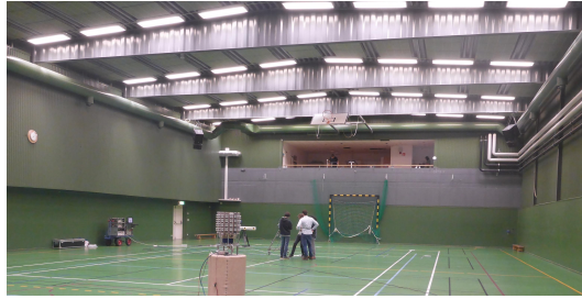
Figure 2: Overview of the measurement area in the sports hall, Medicon Village, Lund, Sweden. Room dimension is around 20\text{ m} \times 36\text{ m} \times 7.5\text{ m} .
