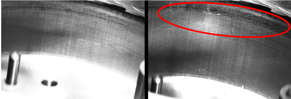
Figure 28 High-speed recording of cylinder liner on running engine, at start and after 30sec running. Encircled the occurring oil droplets and traces.
