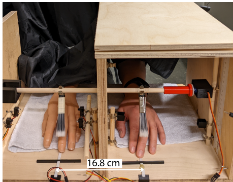
Figure 1: The experimental setup, where brush stroking was applied to the rubber hand and the participant’s hand (classic Rubber Hand Illusion). The white rubber band was used as a guide for where to position the middle finger. The distance between the hands was 16.8 cm.
