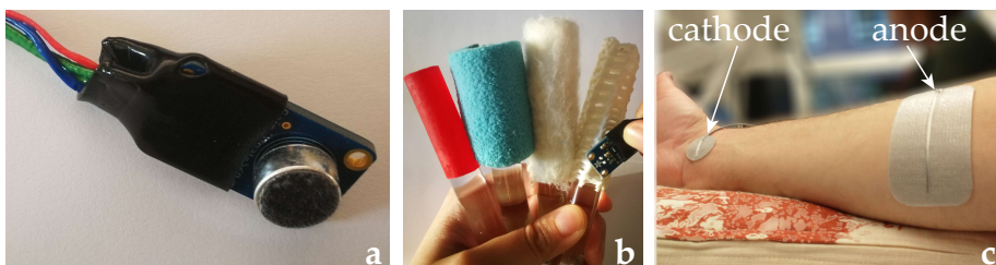
Figure 1. (a) Close-up image of the omnidirectional electret condenser microphone with an amplifier module. An isolation cable was put on the circuit board for an easier grip of the microphone during the stroking and to reduce interference with the components on the printed circuit board (PCB). (b) The experimenter was stroking the different textures with a microphone in a proximal to distal direction. (c) Placement of the electrodes on the participant's forearm. The cathode was placed over the median nerve while the anode was applied on the upper part of the forearm.
