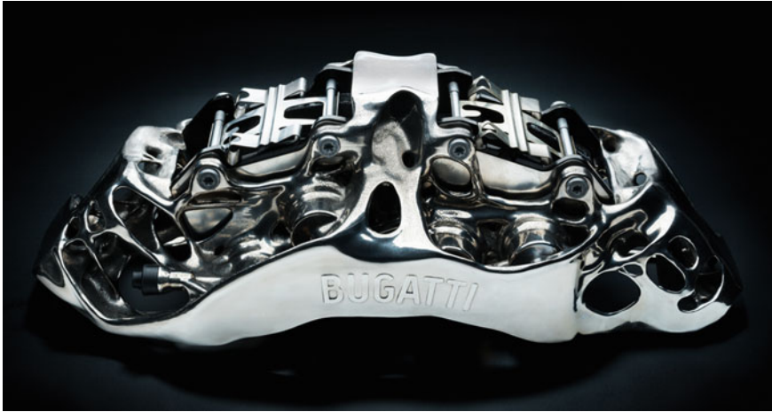
Fig. 6.97 Developed by Bugatti: This eight-piston monobloc brake caliper is the world's first brake caliper to be produced by 3-D printer and also the largest titanium functional component produced by additive manufacturing. ( Image credits (© 2018 Bugatti Automobiles S.A.S.)
