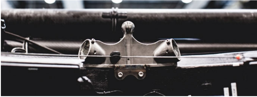
Fig. 6.87 T5 mast ball (Courtesy of Renishaw, credit: Harry KH/INEOS TEAM UK)
