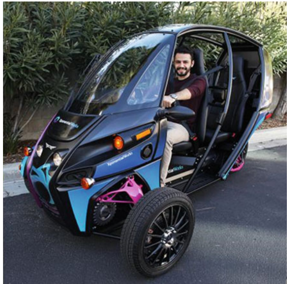
Fig. 6.106 Arcimoto's FUV feature 3D-printed components. The use of 3D printing helped to reduce the weight of the vehicles (Image credits Arcimoto)
