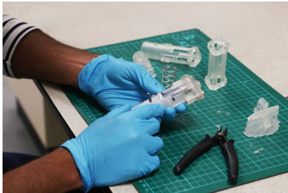
Fig. 6.42 Example of AM medical device (general medical model) for prototyping and testing (Courtesy of Formlabs)
