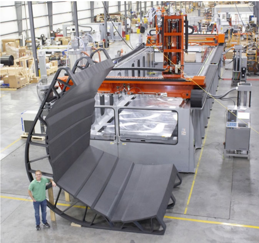
Fig. 6.91 Three-meter section from a 15-m-long yacht hull mold (Courtesy of Thermwood)
