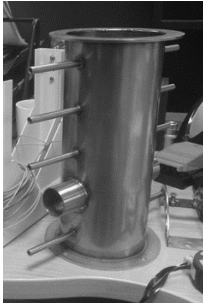
Figure 11 – Photo of modified duct section.
