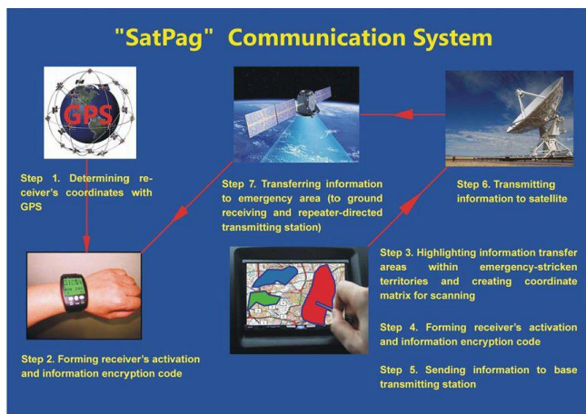
Fig. 3. Using SatPag Professional, information can be sent to different state services in emergency zone.
