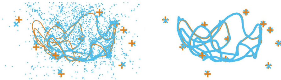
Figure 4: 3D reconstruction (blue) and ground truth (orange) of sound source path from calibration system (left) and from the proposed method (right).
