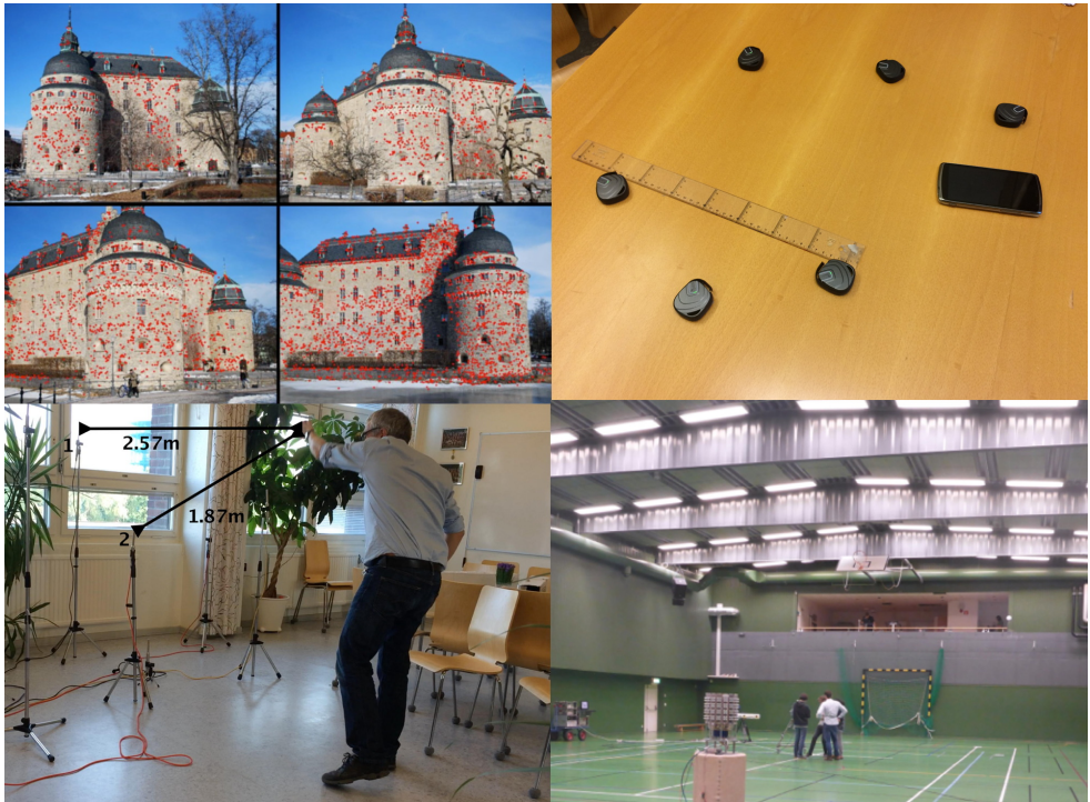
Figure 1: Examples of sensor technologies for map estimation. Top-left: Structure from motion using multiple images, [1]. Top-right: Mobile phones that measure distances to UWB tags, [2]. Bottom-left: Microphones measure difference of distances to ambient sound, [3]. Bottom-right: Massive MIMO units measure distances to radio transmitters, [4].
