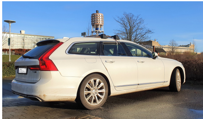
Fig. 2. Photo of array antenna mounted on Volvo V90 Passenger Vehicle.
