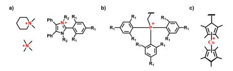
Figure 7. Chemical structures of nitrogen containing cationic groups (a), a nitrogen-free cationic group (b), and an organo metalic cationic group (c).
