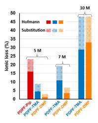
Figure 40 Ionic loss estimated from <sup>1</sup>H NMR spectra of PDPF-Pip, PDPF-TMA and PDPF-DMP via Hofmann elimination and nucleophilic substituiton, respectively.
