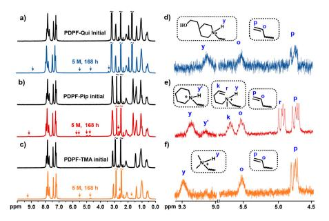
**Figure 29.** <sup>1</sup>H NMR spectra of PDPF-Qui (a), PDPF-Pip (b), and PdPF-TMA (d) were recorded in DMSO-*d<sub>6</sub>*/TFA before and after alkaline treatment with 5 M aq. NaOH at 90 °C for 168 h. The new signals appeared between 4.5-5.8 and 9.0-9.4 ppm after alkaline treatment, 5 M, aq. NaOH at 90 °C for 168 h were indicated by arrows and expended in (d), (e), and (f) panels for PDPF-Qui, PDPF-Pip, and PDPF-TMA, respectively.
