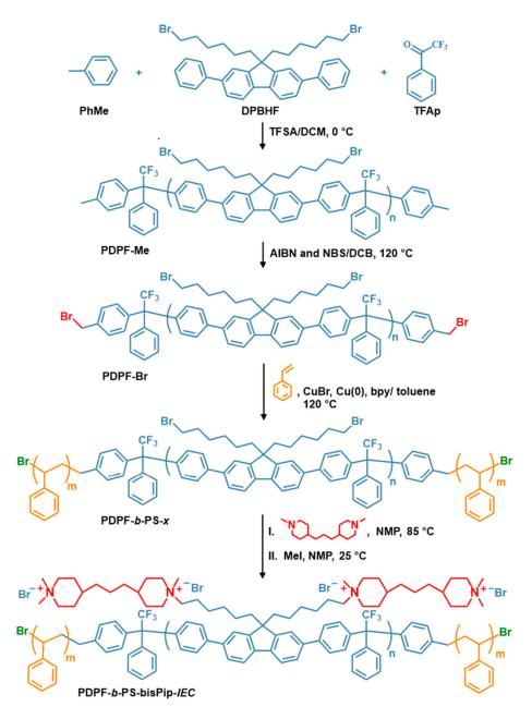
Figure 34. Preparation of the BAB triblock copolymers in four steps: superacid-mediated polyhydroxyalkylation reactions, followed by benzylbromination reaction to generate the macroinitiator. ATPR was then employed to synthesize the polystyrene block, and finally, the midblock was functionalized with dual piperidinium cations to give the PDPF-b-PS-bisPip-*IEC* series.
