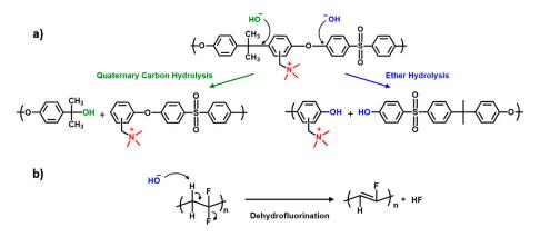
Figure 6. Degradation pathways of polysulfone (a) and polyvinylfluoride (b)( modified from Ladewig et al<sup>53</sup>).
