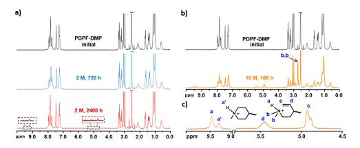
**Figure 39.** <sup>1</sup>H NMR spectra of PDPF-DMP a) before and after alkaline treatment, 2 M aq. NaOH, at 90°C, b) before and after storage in 10 M aq. NaOH, for 168 h, at 90 °C and c) the new signals emerging in the region 4.5-5.7 and 9.0-10 ppm after alkaline treatment 10 M, aq. NaOH, 168 h, at 90°C were expanded.
