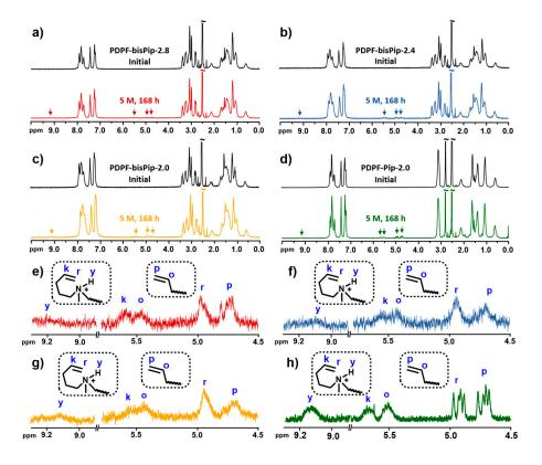
**Figure 32.** <sup>1</sup>H NMR spectra before and after alkaline tratment in 5 M, aq. NaOH during 168 h at 90 °C of a) PDPF-bisPip-2.8, b) PDPF-bisPip-2.4 (c) PDPF-bisPip-2.0 and d) PDPF-Pip-2.0. The signals emerged in the region 4.5-5.7 ppm and 8.8-9.3 ppm after storage in 5 M, aq. NaOH for 168 h at 90 °C are amplified in e) PDPF-bisPip-2.8, f) PDPF-bisPip-2.4, g) PDPF-bisPip-2.0 and h) PDPF-Pip-2.0.
