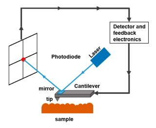
Figure 22. Schematic illustration of the AFM instrument.
