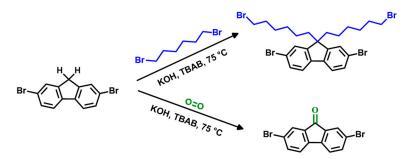
Figure 13. Alkylation reaction of dibromo fluorene with 1.6 dibromohexane<sup>113</sup> (top) and fluorene formation (bottom)<sup>119</sup>.
