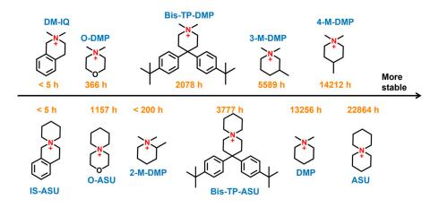
Figure 10. Stability of different QA under  $\lambda$  = 4.8 conditions at 80 °C analyzed by <sup>1</sup>H NMR spectroscopy. Modofief from Lee el at.<sup>55</sup>
