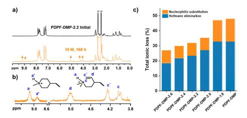
Figure 43. (a) Alkaline stability of the PDPF-DMP-2.2 membane after 168 h storage in 10 M aq. NaOH at 90°C, (b) expansion of the new signal emerged between 3.8-5.8 and 8.6-9.6 ppm , and (c) total ionic loss of the PDPF-DMP-*IEC* series and PDPF-DMP after alkaline treatment in 10 M, aq. NaOH for 168 h at 90°C.
