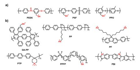
Figure 12. Molecular structure of different functionalized polymers a) arylether-containg polymers and b) aryl ether-free polymer.<sup>54</sup>
