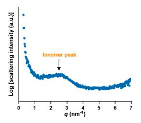
Figure 21. Scattering profile of an AEM with a clear visible ionomer peak
