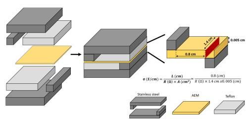
Figure 24. The two-probe cell assembly employed in-plane OH<sup>-</sup> conductivity measurement of the AEM under fully hydrated conditions.
