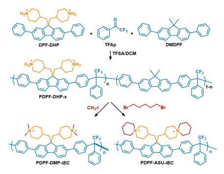
Figure 41. Synthetic pathways to the PDPF-DMP-IEC series of copolymers and and the PDPF-ASU-IEC homopolymer.
