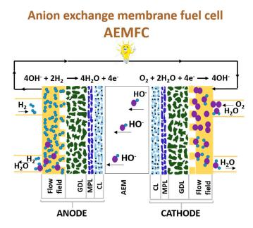
Figure 3. Schematic model of the AEMFC. On both sides there is a of catalyst layer (CL), a microporous layer (MPL), and a gas diffusion layer (GDL).
