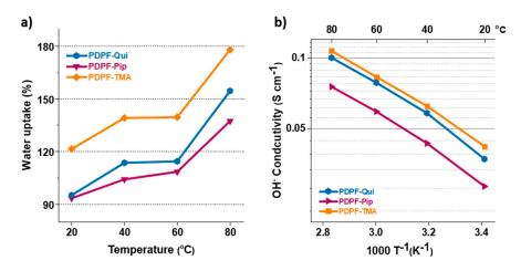
Figure 28. The water uptake of AEMs in the OH<sup>-</sup> form at 20-80 °C (a) and OH<sup>-</sup> conductivity of AEMs as a funtiontion of T<sup>-1</sup> obtained under fully hydrated conditions (b).
