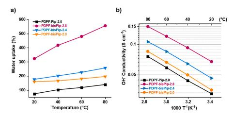
Figure 31. Water uptake of fully hydrated AEMs in hydroxide form as funtion of temperature (a) and OH<sup>-</sup> conductivity of fully hydrated AEMs as a function of  $T^{-1}$ .
