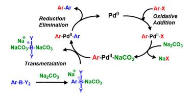
Figure 14. General mechanism for Suzuki coupling reaction between organometallic compounds and organohalides.
