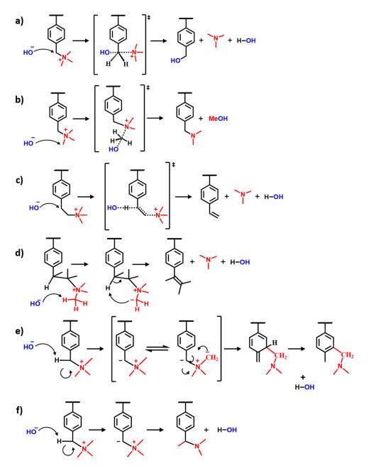
Figure 5. Chemical degradation pathways of QA cations a) nucleophilic substitution at benzyl position, b) nucleophilic substitution at methyl position, c) Hofmann elimination ( $E_2$ ), d)  $E_1$  elimination, e) Sommlet-Hauser rearrangement, and f) Stevens rearrangement.
