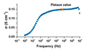
Figure 23. Hydroxide conductivity of the membrane as a function frequency at a constant temperature and a plateau value
