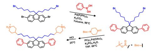
Figure 15. Aryl-aryl Suzuki coupling of aryl-aryl component<sup>113,</sup> (top) and alkyl alkyl Suzuki coupling (bottom).<sup>116</sup>
