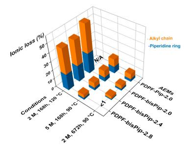
Figure 33. Ionic loss by Hofmann elimination of the AEMs, calculated from <sup>1</sup>H NMR spectra after different alkaline treatments (N/A: not analyzed due to insolubility).
