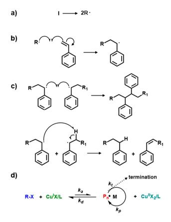
Figure 17. The overall reaction mechanism of the radical polymerization a) initiation, b) propagation, and c) termination. The conventional ATRP mechanism (d), where L and X represent ligand and halogen, respectively.<sup>139</sup>
