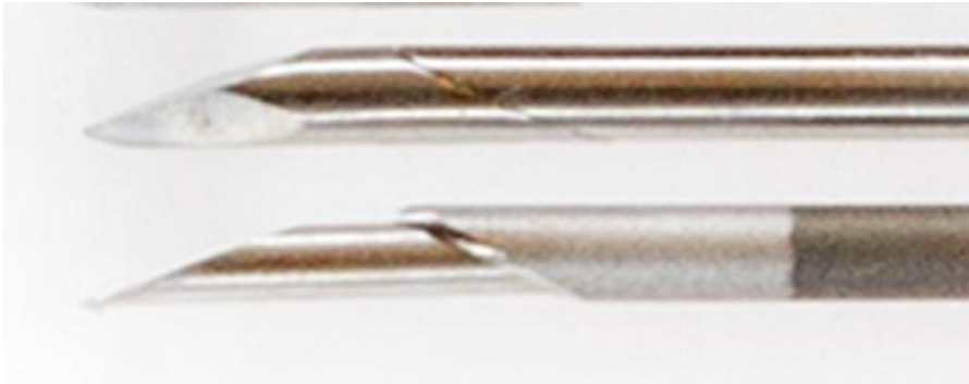
Figure 31 Needle tips: Top: The Forsvall biopsy needle prototype 2 used in Paper 2. Bottom: A Tru-Cut biopsy needle. Photo by Charlotte Carlberg Berg
