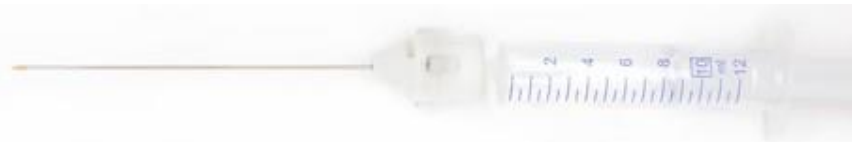
Figure 40 One of the first working prototypes of injection needles, connected to a syringe. Photo by Andreas Forsvall
