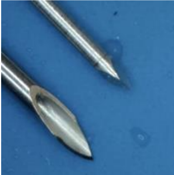
Figure 42 The closed needle tip of the Forsvall injection/aspiration needle and a standard hypodermic needle for reference. Image from microscope. Photo by Andreas Forsvall
