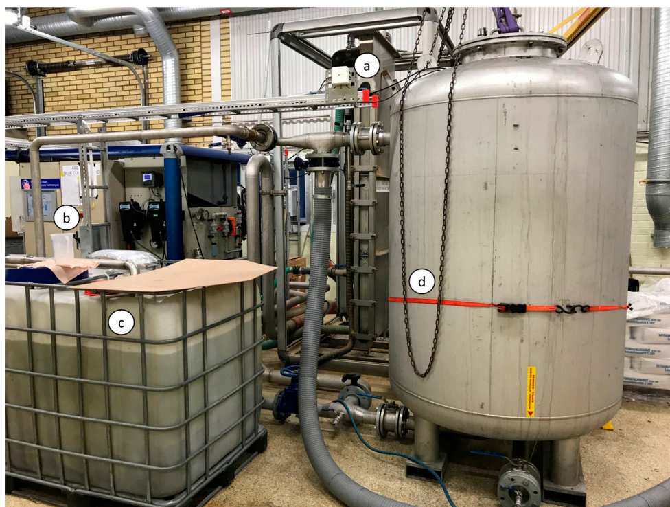
Figure 16. Photograph of the pilot-scale ultrafiltration (UF) and GAC filtration plant described in Paper III, showing the vertical hollow fiber UF membranes (a), control panel and collection tank (b), equalization tank (c), and the GAC filter (d).
