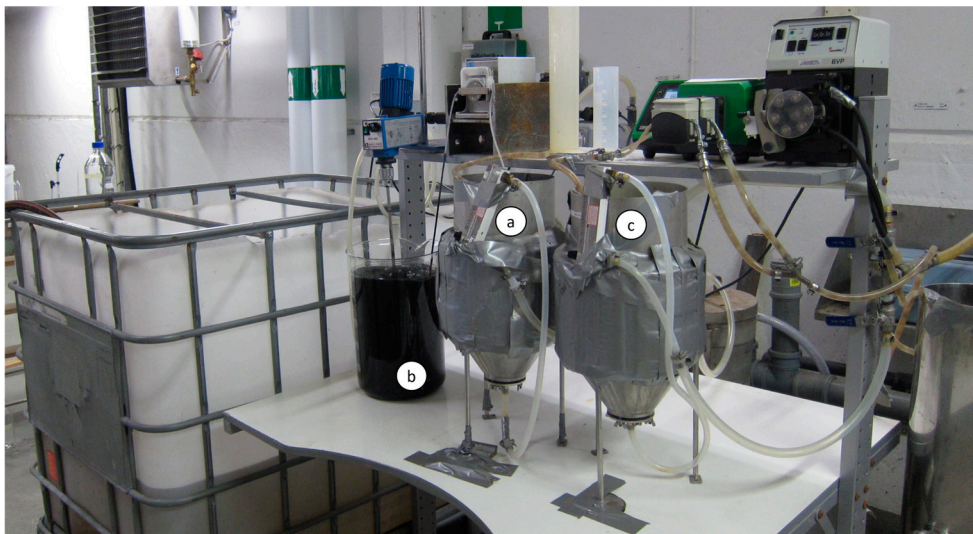
Figure 14. Photograph of the small pilot-scale MBBR units described in Paper IV. Both MBBRs contained nitrifying carriers, and one MBBR (a) was continuously dosed with PAC from a slurry (b), while the other MBBR (c) was not dosed with PAC.
