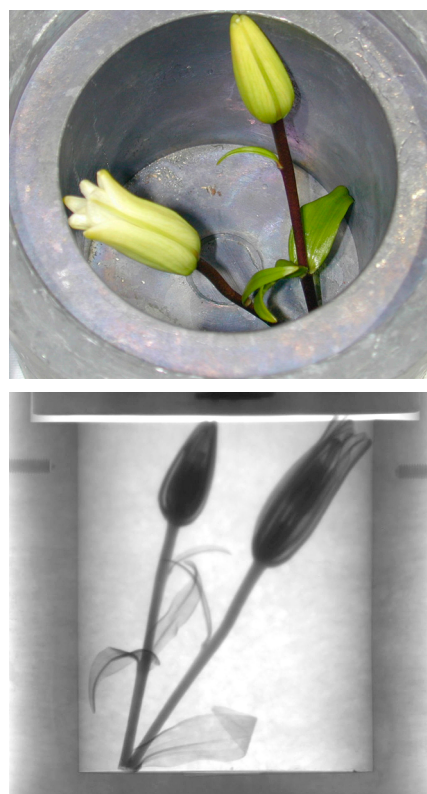
Figure 6. Neutron image of lilies inside a lead cask. The image demonstrates that lead is “transparent” to neutrons, while its sensitivity to hydrogen enable resolving even fine details such as the leaf veins inside the flowers. Image credit: Daniel Hussey/NIST.
