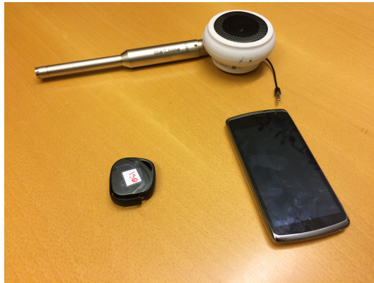
Figure 1: The problem of inferring structure from distance measurements, is relevant for measurements using audio and radio. The top part of the image contains one of the microphones (The t.bone MM1) and one of the speakers used for acoustic experiments. The bottom part of the image contains one ultra-wide-band tag and a ultra-wide-band equipped mobile phone used for radio experiments.
