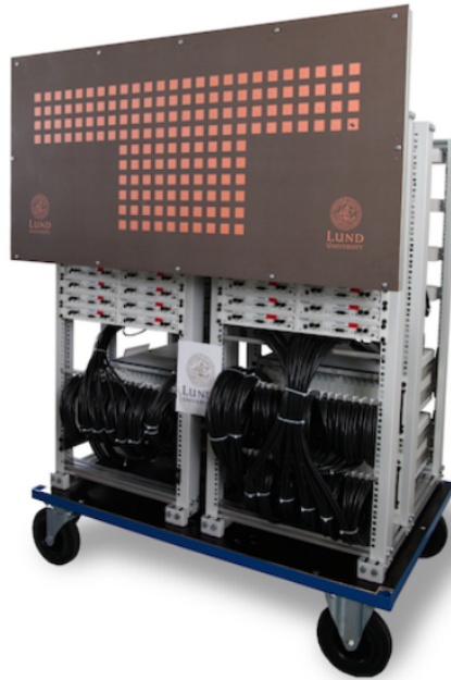
Figure 4.1: The Lund University massive MIMO testbed with the T-shaped array deployed.
