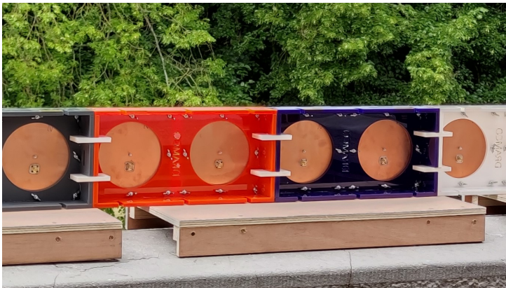
Figure 3: Multiple modular antenna holders connected.
