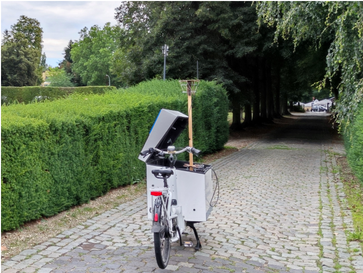
Figure 2: Transmit node with a single dipole antenna.
