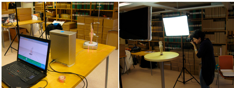
Figure 3.8 3D digital data acquisition with a laser scanner (left) and image-based 3D modelling technique (right) at Gastelyckan – LUHM (Vassallo©).
