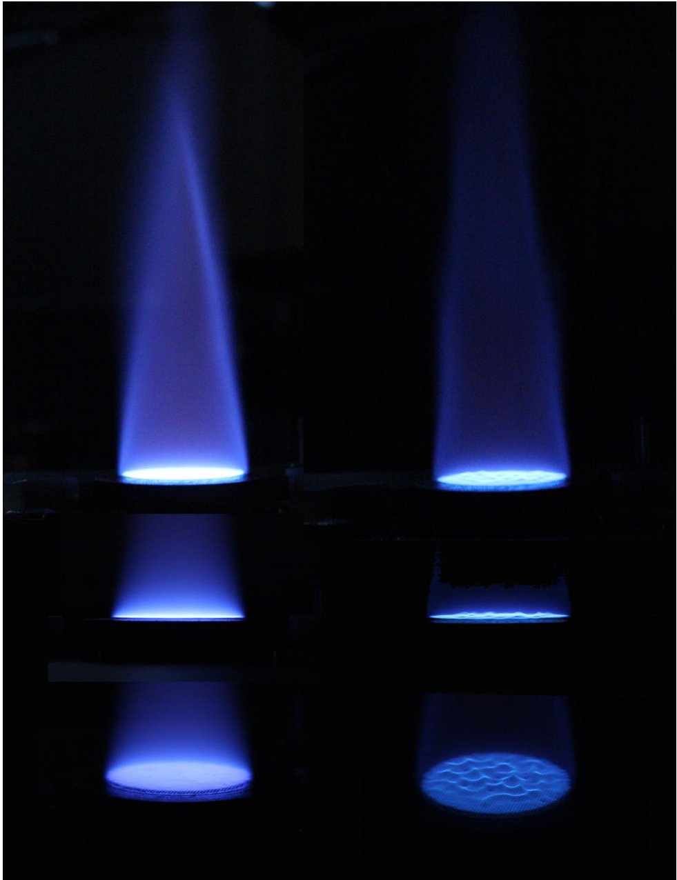
Figure 3: The pictures at the left show the flame front of a flat flame and the pictures at the right the flame front of a corrugated flame. Both flames are shown from the side as well as from above at an angle. The cone above the flames represents in each case the post flame zone. The flames in the pictures are ethanol+air flames mounted on a Heat flux burner.
