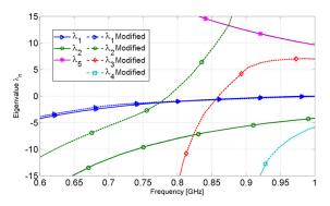
Fig. 1. Characteristic eigenvalues of a 130 mm  $\times$  66 mm chassis with and without shorted metal strips along the longer ends.
