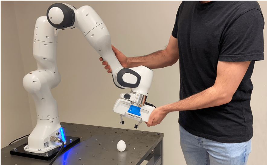
Figure 1. Setup for the kinesthetic teaching task described in Sec. 4.2. A Franka Emika Panda robot is mounted on a table. The blue piece allows to attach a camera to the robot’s end effector. The human operator is manually guiding the robot and displacing it away from its original trajectory and arbitrarily close to the object of interest, here, an egg.
