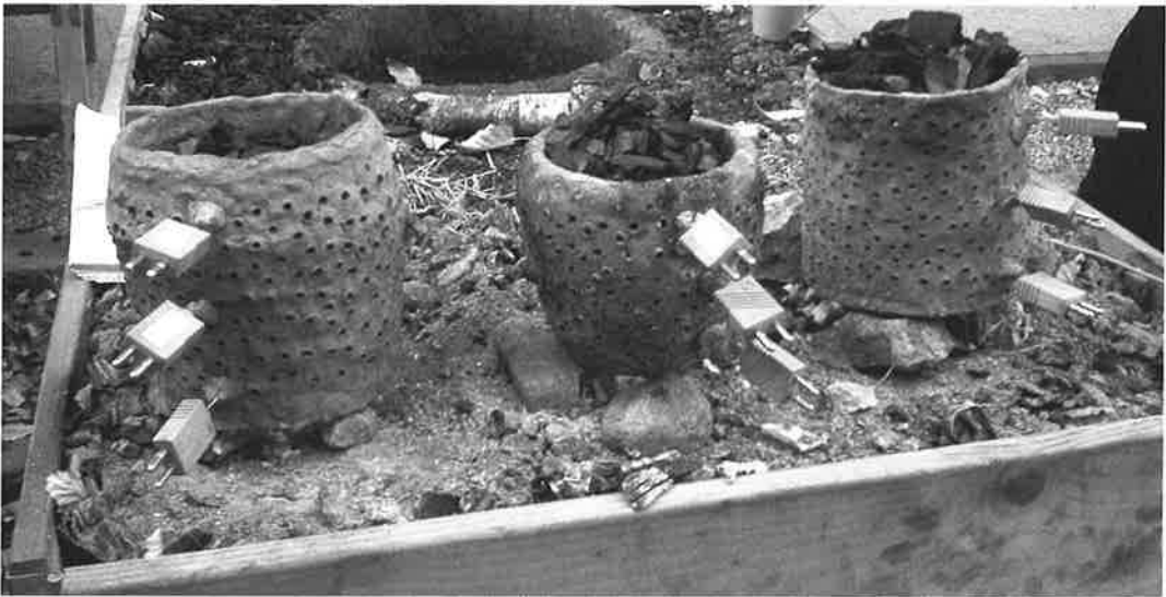
Fig. 3. During the experiments the temperature in the cylinders was measured at three different levels.
