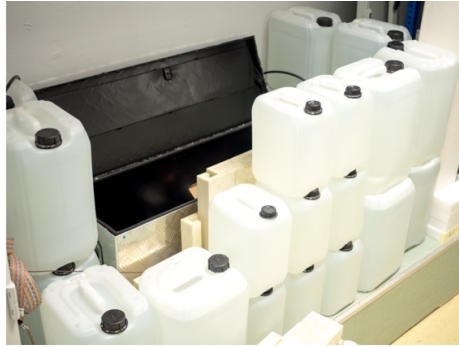
Figure 4: The black-box at the STF. On the left, a CAD drawing of the apparatus under construction and on the right, a photo of the existing prototype. The light-tight box may be surrounded by modular shielding.
