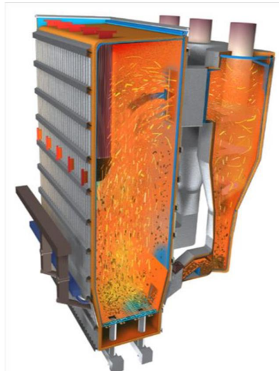
Figure 1.5: Illustration of the loop in circulating fluidized bed furnace [21]. The figure is reproduced with permission from the publisher.
