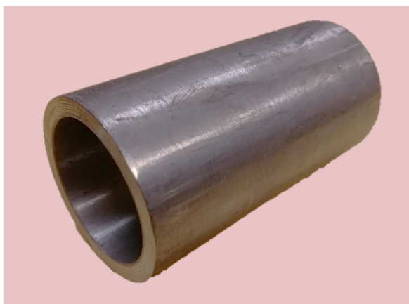
Figure 4.6 Rose metal shield for intratherapeutic preclinical PET imaging.
