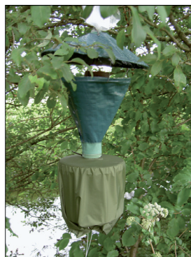
Figure 2. A J alas moth trap. The bait container was filled with wine-based or beer-based bait. Attracted insects fall into the lower compartment where they remain until the trap is checked..
