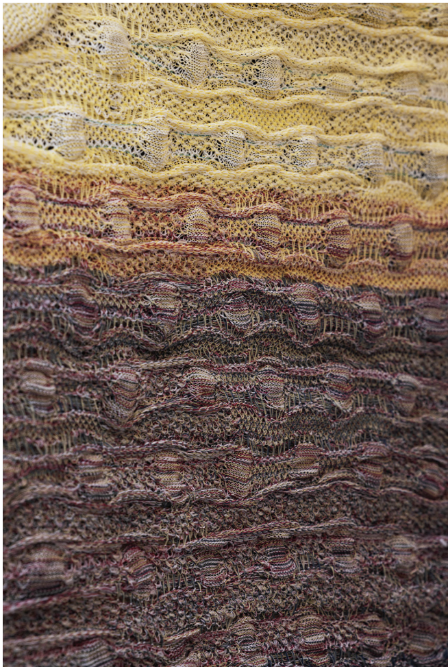
10 As well as providing color, tactility, and enhancing acoustics, the knitted textile provides a filter over the channel openings
