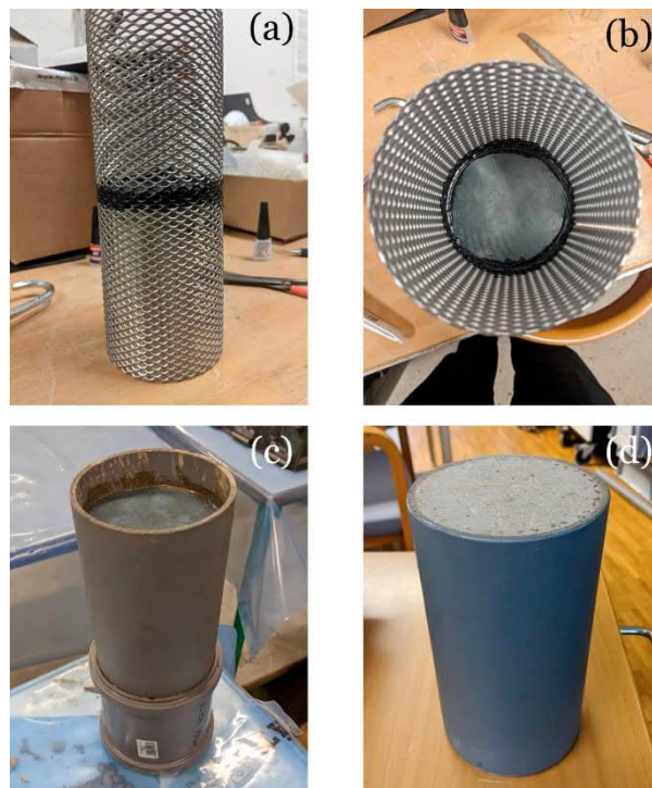
Figure 5. (a) Side-view of the expanded metal cylinder with the OK-plate attached to it. (b) Top-down view of the cylinder in (a). (c) Concrete cylinder immediately after casting. The total length of the concrete cylinder is here 250 mm, but the PVC pipe is longer. (d) Shows a concrete cylinder after being cut to length of 200 mm.
