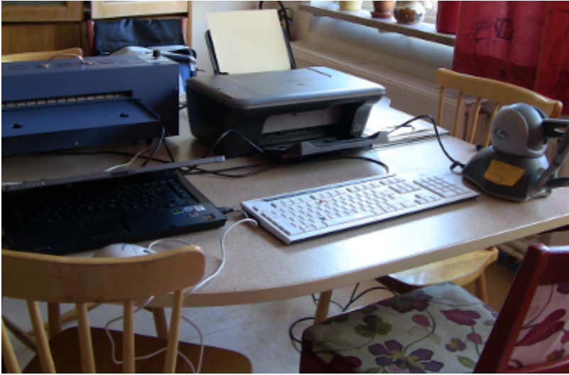
Figure 15: Physicality of the HIPP system, with printer and swelling machine alongside the computer and haptic pen.
