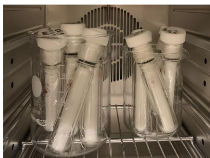
Figure 13. Photo of containers used in alkaline stability evaluations placed inside an oven.
