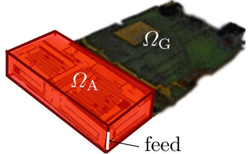
Figure 1. Example of a region  $\Omega = \Omega_A \cup \Omega_G$  decomposed into an antenna design region  $\Omega_A$  and a surrounding fixed region (ground plane)  $\Omega_G$ . The desired feed point is indicated.
