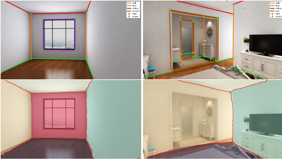
Figure 1: The images on top show the desired results from Semantic Room Wireframe detection and below are the results from a Room Layout estimation algorithm [1]. Lines are added between all detected planes for comparison. The algorithm produces satisfying results on simple scenes (left) but is lacking on more complex scenes, e.g. to the right where the wide opening is erroneously classified as part of the wall.
