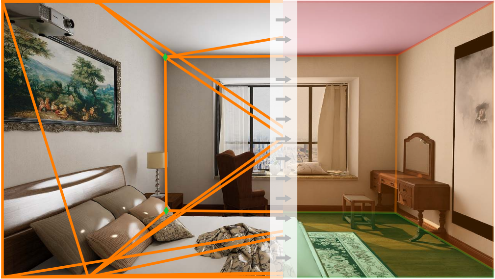
Figure 4.3: The proposed model in Paper III takes an image and a wireframe to produce a set of polygons corresponding to a Room Layout.
