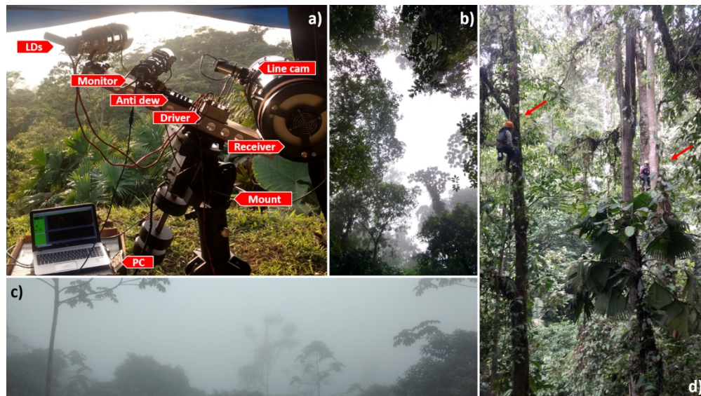
Fig. 1. a) Entomological-lidar system and its main components overlooking the Jardin de los sueños private forest, during a clear moment (17:30). b) Photo displaying the top of canopies at ~30 m over ground disappearing into the mist (9:30), c) A view from lidar toward valley at noon (12:05), typical of the field campaign days. The mist is impenetrable. d) Ecological studies in tropical virgin forests are challenging due to topography, tall vegetation structure, and stratification of ecological niches, here two chiroptologists install a bat net 20 m above ground.
