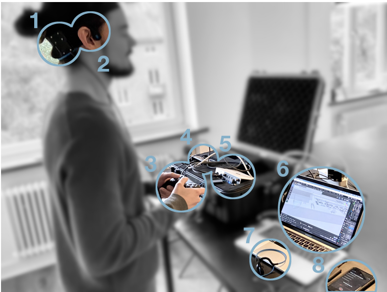
Fig. 5.2: Virtual reality system, Parrot-VR, test setup: 1) inertial measurement unit; 2) bone-conductive headphones; 3) controller; and 4) embedded computer. Auxiliary equipment: 5) audio interface; 6) laptop; 7) bone-conductive headphones; and 8) audio recording device. Figure and caption reprinted from [163].
