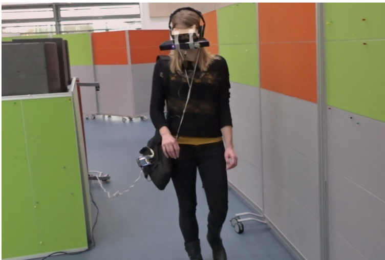
Fig. 7.3: Test of the first Audomni prototype. Note that it was not battery-powered, and only worked indoors.
