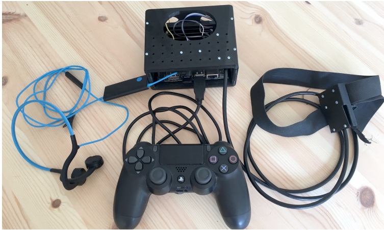
Fig. 5.1: Virtual reality system, Parrot-VR, hardware. Clockwise from left: bone-conductive headphones; embedded computer and audio interface; headband with inertial measurement unit; controller. Figure and caption reprinted from [163].
