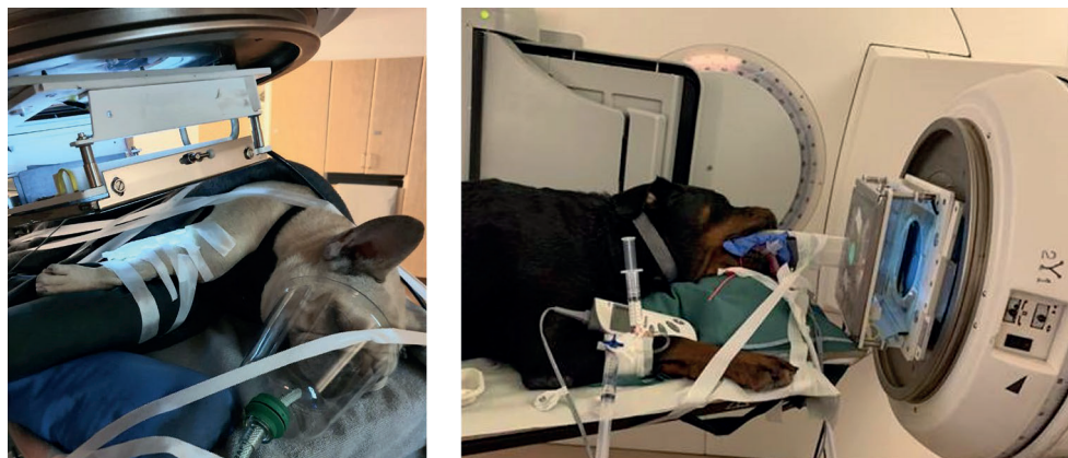
Figure 13: Two examples of treatment setups for FLASH radiotherapy of canine cancer patients at the modified clinical linear accelerator.
