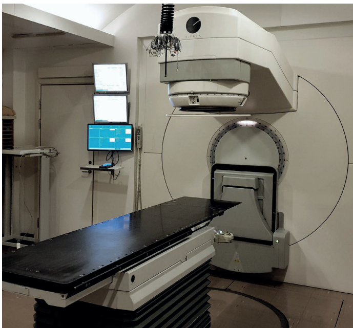
Figure 4: Photograph of the Elekta Precise linear accelerator modified for ultra-high dose rate delivery, which is used in the work throughout this thesis.
