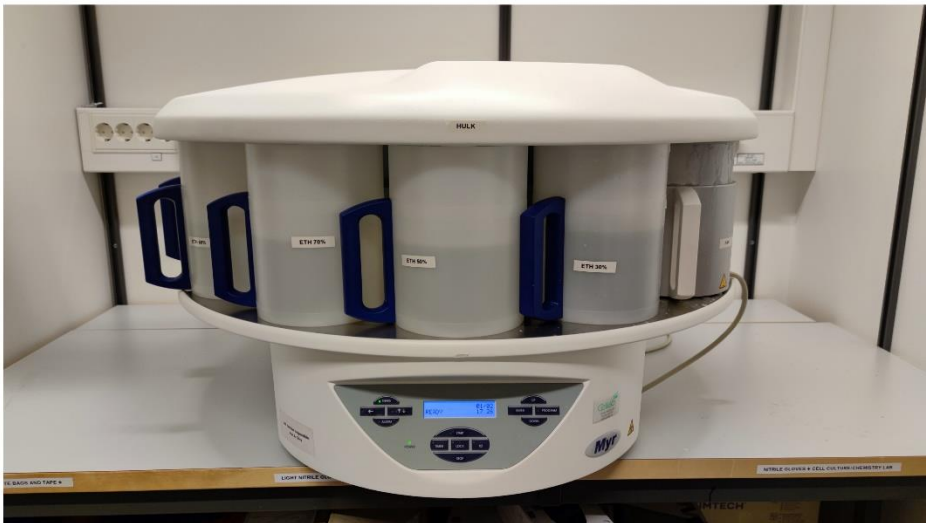
Figure 10 Spin Tissue Processor STP 120 showing individual containers 1-12 and the programmable interface.
