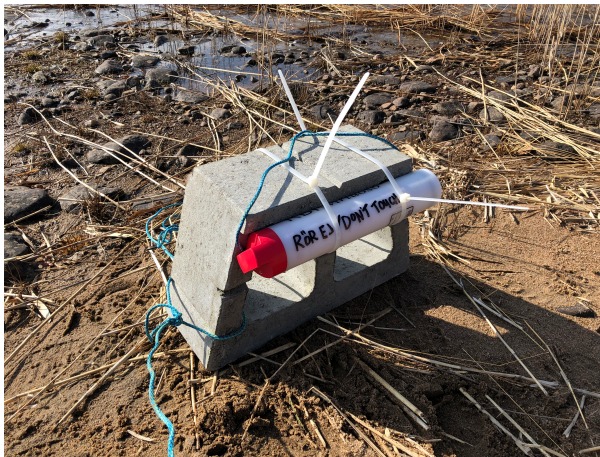
Figure 10: Pressure gauge as deployed in Lake Bolmen. The concrete block ensures a stable locations of the pressure gauge and keeps it above the lake bottom to prevent debris and fine sediment to block the pressure membrane.
