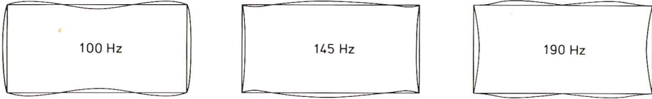
Figure 5.15. Vibration shapes for 1 mm steel sheet
