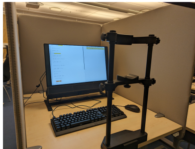
Figure 11: The experimental setup. The apparatus is contained within a booth, with the eye-tracker visible below the screen and a chin- and forehead rest in the foreground.
