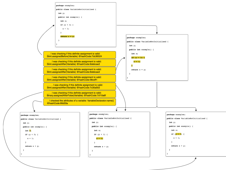
Figure 11: The error trace details shown in order of occurrence in the computation with arrows pointing to how the highlighting in the code changes on hover over error details.
