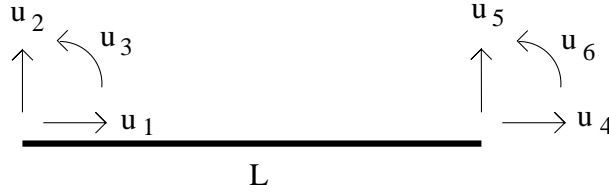
Figure 6.1: Straight beam element with degrees of freedom u_1 \dots u_6 .
