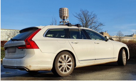
Fig. 2. The massive antenna array on top of the measurement vehicle.
