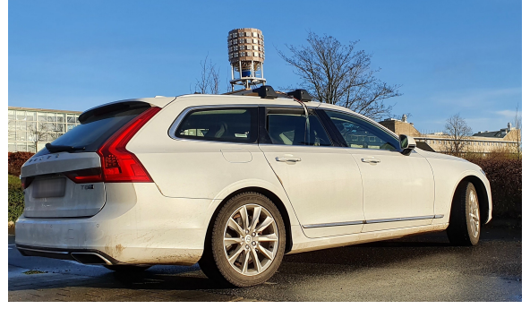
Fig. 1: The massive antenna array on top of the measurement vehicle [13].
