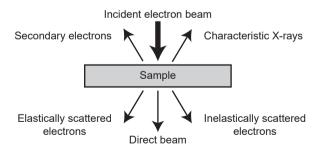
Figure 3.3: A schematic detailing some of the signals generated when the electron beam interacts with a sample.
