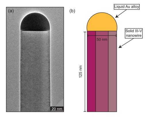
Figure 1.1: (a) An electron micrograph of a nanowire. (b) A schematic representation of the nanowire shown in (a), highlighting the nanoparticle, the solid nanowire and the dimensions. Note that the dimensions are only typical and might vary depending on how the nanowire was grown. In this case, the end of the nanowire is not depicted and extends several hundred nanometers outside of the figure.
