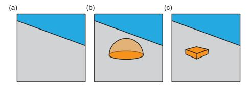
Figure 2.3: (a) A supersaturated vapor phase, now with a substrate surface present. (b) An isotropic nucleus has formed at the substrate-vapor interface. (c) An anisotropic nucleus has formed at the substrate-vapor interface.
