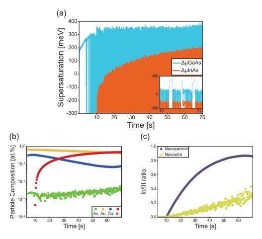
Figure 5.6: Simulation results of the evolution of Au-seeded InGaAs nanowires, grown from GaAs stems. The In supply was initiated at t = 10 s. (a) The supersaturation of GaAs and InAs. The inset shows the same range, but for a magnified timescale. (b) The nanoparticle composition. (c) The nanoparticle and nanowire In/III ratios. The data in (b) and (c) are plotted for nucleations, while the data in (a) is plotted in a continuous manner.
