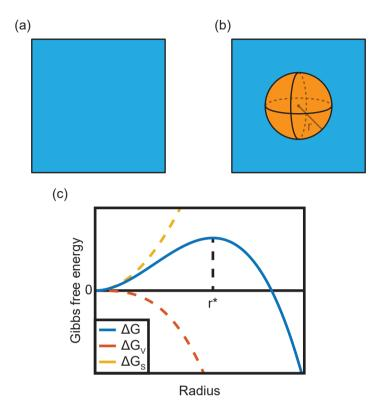
Figure 2.2: (a) Schematic illustration of an infinite vapor phase without walls or borders (you might have to use your imagination for this one). (b) A liquid nucleus with radius r has formed in the supersaturated infinite vapor phase. (c) A schematic representation of the difference in Gibbs free energy as a function of radius, along with the volume associated term and the surface associated term. The critical radius for stable growth, r\* is marked in the graph.
