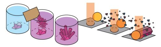
Figure 1: English: Left: The growth of a crystal from a commercial crystal growth kit for children. Right: The growth of a nanowire while it is being illuminated by an electron beam.
