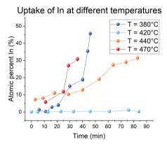
Figure 4.3: Study of the In incorporation in Au nanoparticles at different temperatures. As can be seen, the trend for T = 380°C shows the steepest increase of In concentration over time, while T = 420°C results in little to no incorporation. Gas supply was initiated at time = 0 min.
