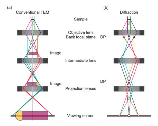
Figure 3.4: Schematics illustrating the beam path while operating the transmission electron microscope in parallel beam mode for conventional TEM imaging (a) and diffraction (b). The main difference between the two configurations is the strength of the intermediate lens, which decides what information will be conveyed to the projection lens system.
