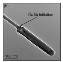
Figure 4.2: Two cases of GaSb growth from GaAs stems. (a) Early GaSb growth before growth parameter optimization. (b) GaSb growth after growth parameter optimization.
