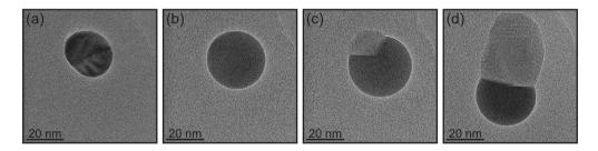
Figure 4.1: A nucleation event observed in the environmental transmission electron microscope. (a) A solid Au nanoparticle residing on a substrate. (b) The nanoparticle is now liquid due to alloying with growth species at elevated temperatures. (c) The nucleus has formed and the nanoparticle is wetting several facets. (d) The crystal is starting to look like a nanowire, as the nanoparticle has decided on a facet for the continued growth.
