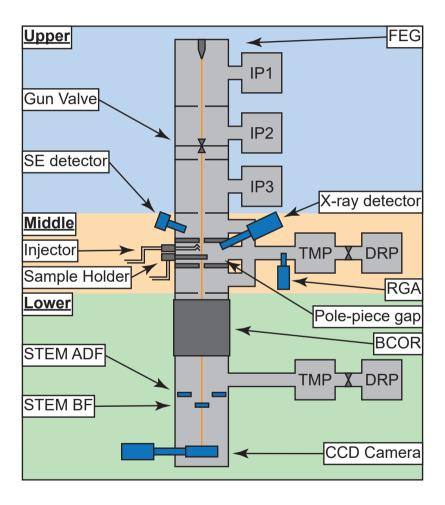
**Figure 3.7:** A schematic of the environmental transmission electron microscope at Lund University. The schematic is splitting the microscope into three parts: Upper, middle and lower.
