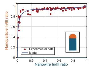
Figure 5.3: The compositional relationship between nanoparticle and nanowire for Au-seeded InGaAs. The y-axis shows the In/III ratio for the nanoparticle, while the x-axis shows the In/III ratio for the nanowire, color coded similarly to the schematic inset. In the graph, both experimental data (red circles) as well as model results (blue line) are shown. Figure adapted from Paper π
