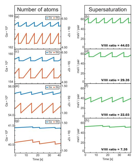
Figure 6.5: Further data extracted from four of the GaSb simulations. The graphs show how the number of atoms for Ga and Sb and the supersaturation changes over time for a subset of the simulations (full length is 300 s). The cases are from the TMSb flow series, spanning V/III ratios of 44.03 (a)-(b), 29.35 (c)-(d), 22.03 (e)-(f) and 7.35 (g)-(h).
