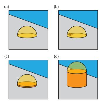
Figure 2.5: (a) A liquid seed particle residing on a substrate surface. (b) A nucleus has formed within the droplet, at the substrate-droplet interface. (c) The nucleus has grown to cover the whole interface. (d) The nanowire has started to grow vertically from the surface.
