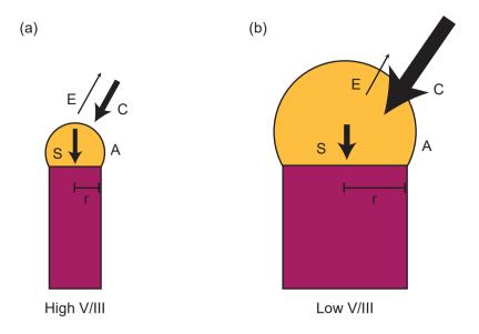
Figure 6.6: A schematic detailing atomistic pathways in the model. (a) A high V/III ratio case. (b) A low V/III ratio case. In the figure, E stands for evaporation, C for condensation, S for solidification, A for the surface area of the nanoparticle and r indicates the nanowire radius.
