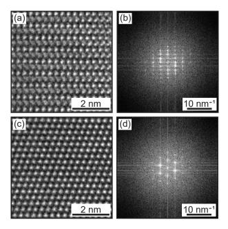
Figure 4.8: FFT patterns of crystal structures. (a) A segment of WZ imaged using HRTEM, with its corresponding FFT shown in (b). (c) A segment of ZB imaged using HRTEM, with its corresponding FFT shown in (d).
