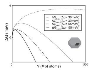
**Figure 6.8:** A model illustrating the nucleation of twinned and non-twinned layers of GaAs. The change in Gibbs free energy is plotted as a function of number of atoms for different supersaturations. The inset illustrates the assumed shape of the nucleus on the top facet. Figure adapted from **Paper v**.
