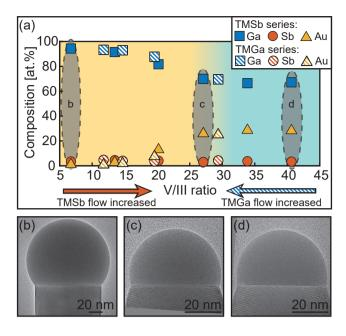
Figure 5.1: Au-based nanoparticle composition and size depending on the supplied V/III ratio, for Au seeded GaSb nanowires.
