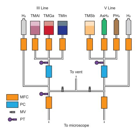
Figure 3.9: A schematic of a simplified view of the GHS used in connection to the environmental transmission electron microscope. Most importantly, the split between the group III and group V line, and the point where they meet, is illustrated. The H<sub>2</sub> lines that enter each bubbler separately have been omitted for clarity.
