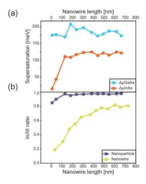
Figure 5.5: A study of the evolution of a nanowire as it is growing, presented as a function of the grown length. (a) The supersaturation of GaAs and InAs. (b) The In/III ratios measured in the nanoparticle and nanowire.
