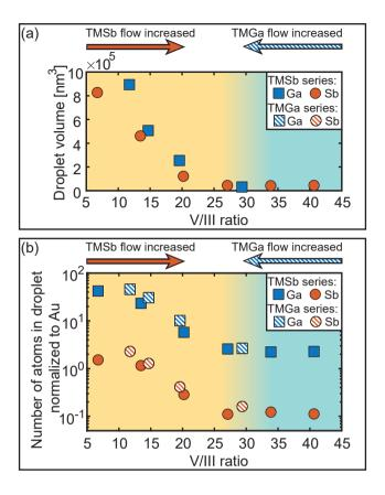
Figure 6.2: (a) The volume of the nanoparticle as a function of V/III ratio for Au-seeded GaSb growth. (b) A recalculation from concentration to number of atoms dissolved in the nanoparticle. The values are normalized to the amount of Au. The graphs are color coded based on the aforementioned stable (cyan) and dynamic (yellow) diameter and composition regimes.
