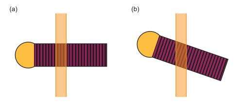
Figure 4.6: Schematic of nanowire illumination during the XEDS acquisition, detailing an on-axis nanowire (a) and a tilted nanowire (b). The nanowire is striped to illustrate the atomic layers. In (a), four purple lines are illuminated, while in (b) six different purple lines are partially illuminated. This illustrates that the XEDS information will be more localized if the nanowire is illuminated on-axis.
