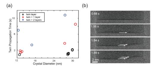
Figure 6.9: Multiple nucleation events observed in conjunction with the formation of twins in GaAs. (a) A collection of several observations where one or two layers nucleate before the twinned layer is completed, for various investigated nanowire diameters. (b) One such example, where the arrows point to the growth fronts of the individual layers and the time stamp is related to Movie S3 in the original publication. Figure adapted from Paper v.
