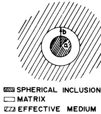
Figure 4: Generalised self-consistent scheme, sphere with a concentric shell of matrix material in an effective medium.
