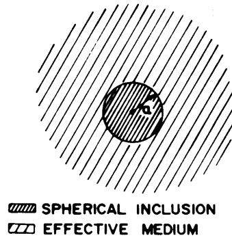
Figure 3: Self-consistent scheme, sphere in an effective medium.
