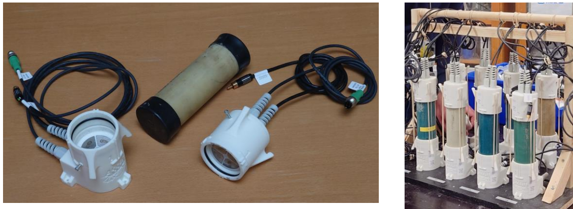
Figure 2 Photographs showing electrode lid design for the piece-of-pie shaped electrodes together with sample cylinder with standard lids (left), and a group of lab samples prepared for measurements (right).
