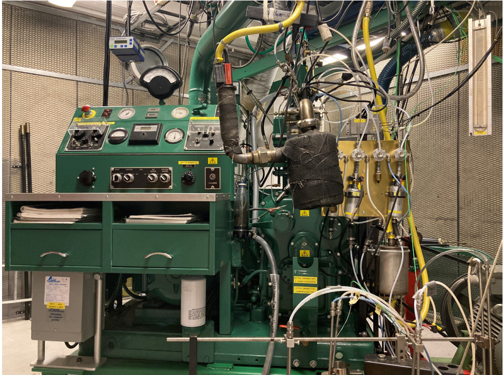
Fig. 3.2. The modified CFR engine at the Energy sciences lab of Lund university.
