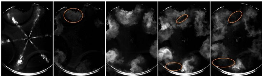
**Figure 5.12.** Different stages of combustion process inside the wave piston
