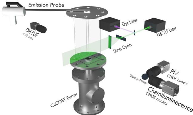
**Figure 5.15.** Schematic illustration of gas turbine burner setup
