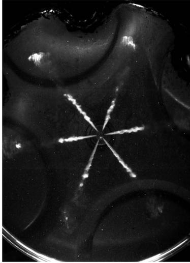
**Figure 2.2.** Natural Fuel spray visualization with high-speed imaging of Mie scattering in optical engine.
