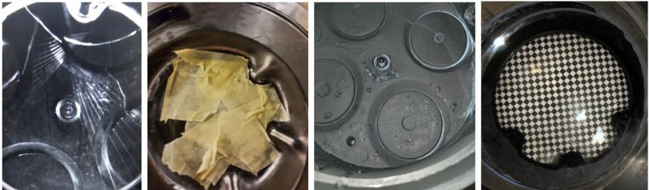
**Figure 5.9.** A view of the wave piston reflections (left) and sprayed surface (middle) and resulted FOV (right)
