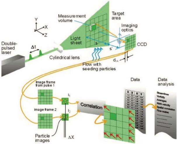
Figure 4.4. A schematic representation of a PIV measurement [9]
