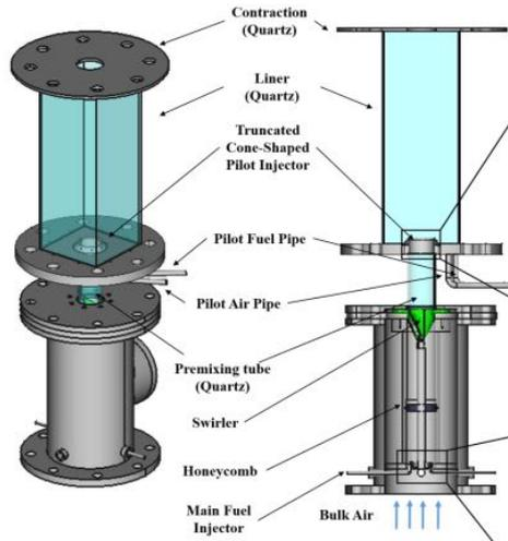
**Figure 3.3.** CeCOST gas turbine combustor model [20]
