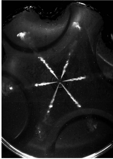
Figure 2.2. Natural Fuel spray visualization with high-speed imaging of Mie scattering in optical engine.
