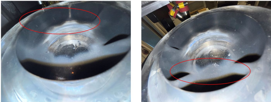
Figure 5.14. Distinctions of soot accumulation pattern in wave side and non-wave side in higher engine loads
