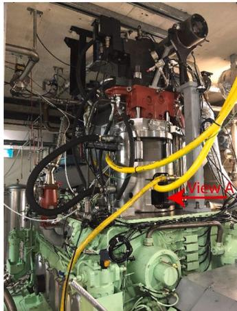
**Figure 5.4.** Optical Engine based on Wärtsilä W20DF marine engine
