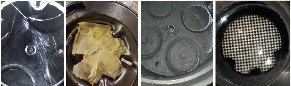
Figure 5.9. A view of the wave piston reflections (left) and sprayed surface (middle) and resulted FOV (right)
