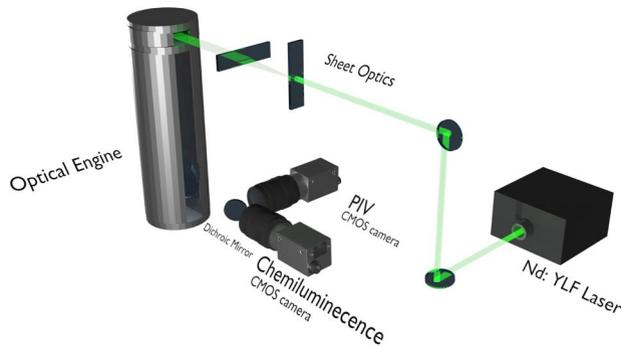
**Figure 3.1.** Heavy-duty optical engine, Volvo MD13, and PIV-FIV experimental setup (top), Schematic illustration of the setup (bottom)
