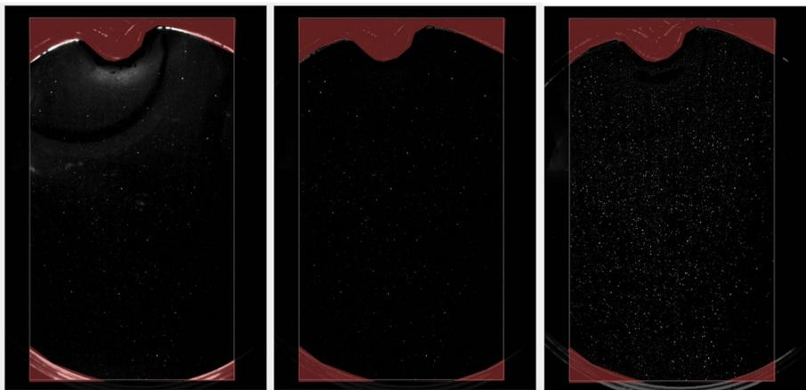
**Figure 4.2.** Image pre-processing for PIV, raw image(left), high pass filtered (middle) and intensity capped (right)
